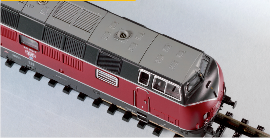
Replication of the first series roof design
